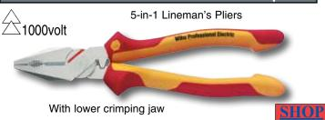
32821 Insulated Lineman's Pliers "5-in-1" Professional Design Insulation According to EN/IEC, ASTM, NFPA70E & CSA,  $\stackrel{}{\sim}$  up to 1000 Volt. Individually Tested. Deep cut radius conduit jaws for non-slip griping. Extra long induction hardened precision matched cutting edges. Lower crimping jaw accepts most standard non-insulated electrical connectors. Large head with square anvil surface on each side. Made from premium C70 tool steel forgings. 64HRC cutting edges.
