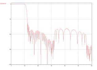
Figure 79 DAC Filter Response 22.05k Sample Rate
