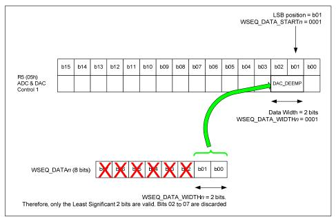
Figure 74 Control Write Sequencer Example
