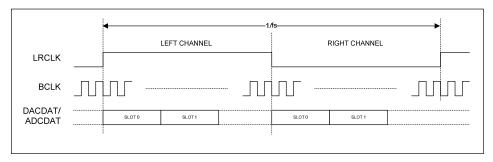
Figure 52 TDM in Left-Justified Mode
