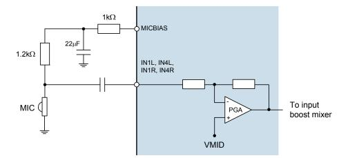
Figure 97 Microphone Connection, with MICBIAS filter components
