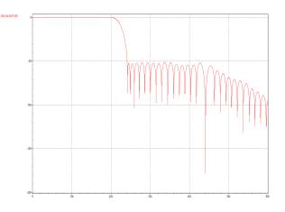
Figure 82 DAC Playback Filter Response for 44.1k Sample Rate
