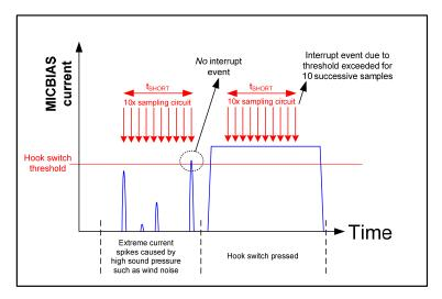
Figure 17 MICBIAS Hook Switch Detection Filtering
