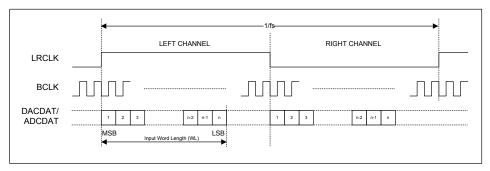
Figure 45 Left Justified Audio Interface (assuming n-bit word length)
