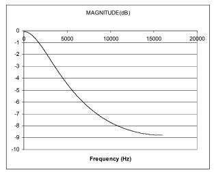
Figure 89 De-Emphasis Digital Filter Response (32kHz)
