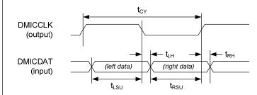
Figure 2 Digital Microphone Interface Timing
