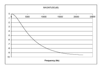
Figure 91 De-Emphasis Digital Filter Response (44.1kHz)
