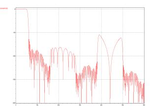
Figure 76 DAC Filter Response for 11.025k Sample Rate
