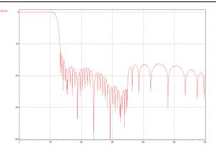
Figure 80 DAC Playback Filter Response for 24k Sample Rate
