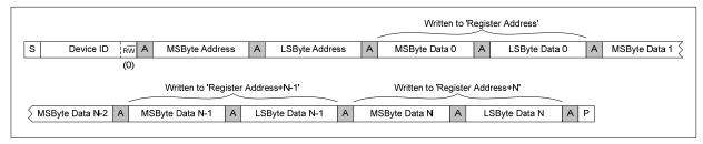
Figure 68 Multiple Register Write to Specified Address using Auto-increment
