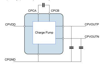
Figure 38 Charge Pump External Connections
