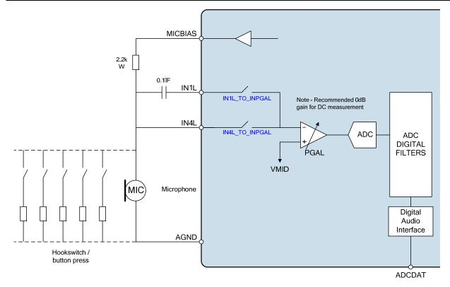
Figure 18 Multiple Hook Switch Detection
