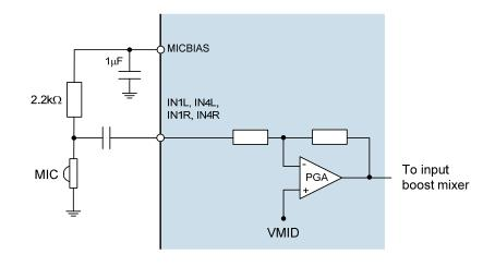
Figure 96 Single Ended Microphone Connection
