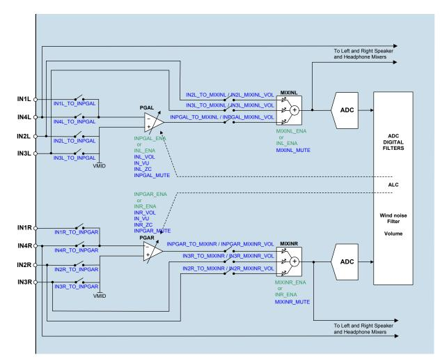
Figure 13 Analogue Input Signal Path
