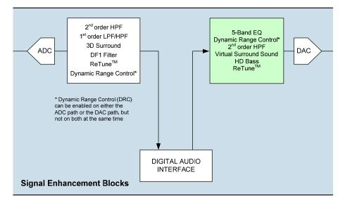
Figure 32 DAC Signal Enhancements
