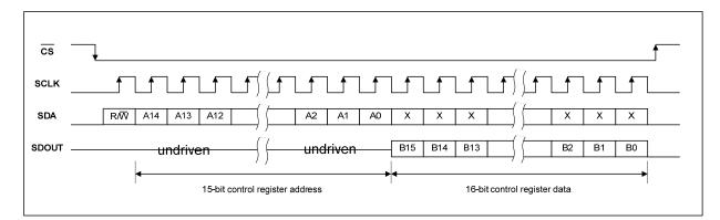
Figure 73 4-Wire Readback (Wired-'OR')
