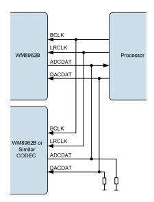
Figure 43 TDM with Processor as Master
