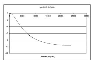
Figure 93 De-Emphasis Digital Filter Response (48kHz)
