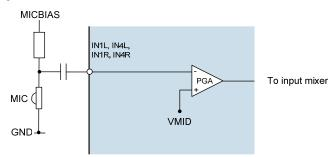
Figure 14 Microphone Input IN1 or IN4
