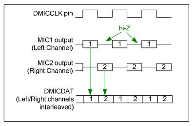
Figure 22 Digital Microphone Interface Timing
