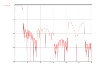
Figure 77 DAC Filter Response for 12k Sample Rate
