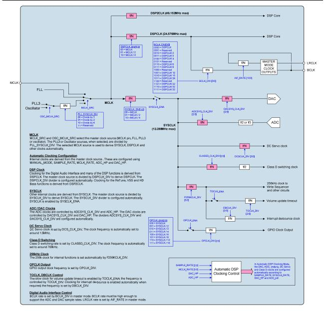
Figure 58 SYSCLK and Internal Clocking Scheme
