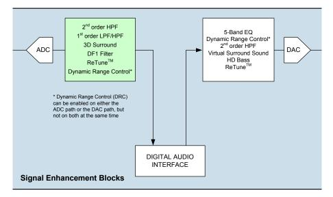
Figure 23 ADC Signal Path Enhancements
