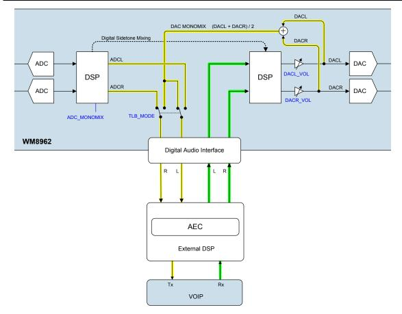
Figure 31 T-Loopback Signal Paths
