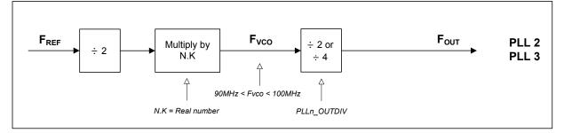
Figure 62 PLL Frequency Control
