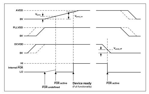
Figure 12 Power On Reset Timing - DCVDD Enabled First
