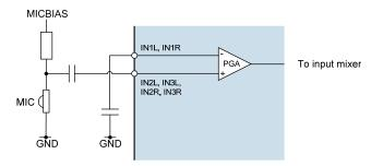
Figure 15 Microphone Input IN2 or IN3
