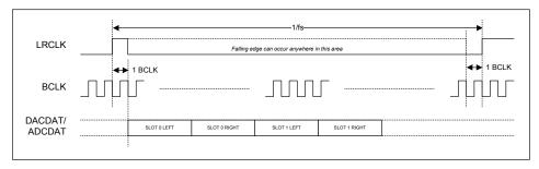
Figure 54 TDM in DSP Mode A
