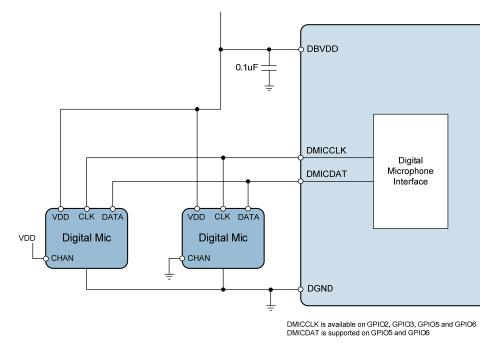
Figure 21 Digital Microphone Input
