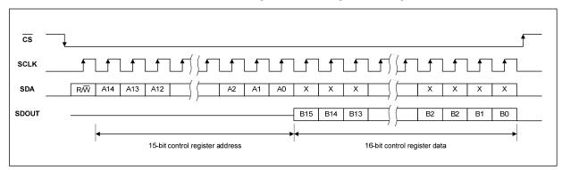
The 4-wire control mode timing is illustrated in Figure 72 and Figure 73.
