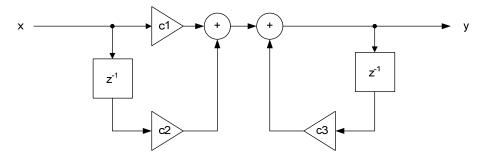
Figure 27 Direct-Form 1 Standard Filter Structure
