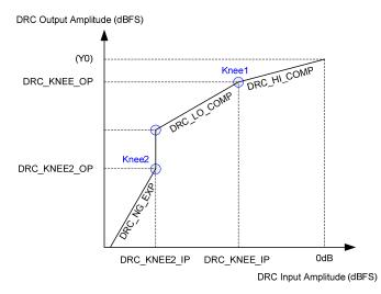
Figure 29 DRC Response Characteristic
