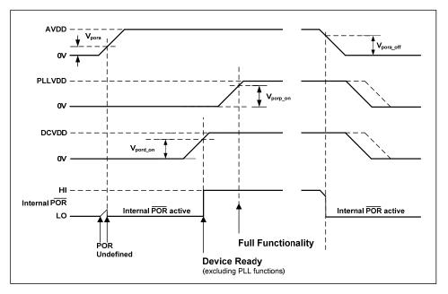
Figure 11 Power On Reset Timing - AVDD Enabled First
