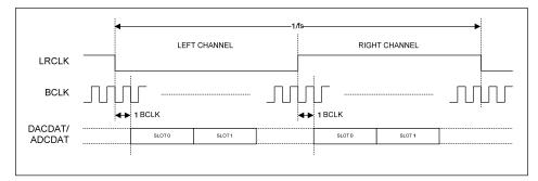
Figure 53 TDM in I<sup>2</sup>S Mode
