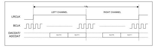
Figure 51 TDM in Right-Justified Mode
