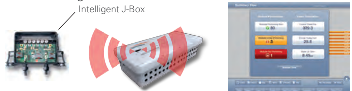
PV panel performance data send to Active Combiner
