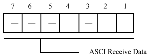
Figure 31. ASCII Receive Register Channel 1R
