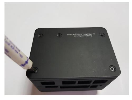
8. In case no Antenna usage, Use the SMA rubber to cover the SMA hole.
