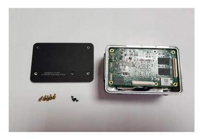
2. Fasten the UPCP PCB on top cover by 2 different kinds of hex standoffs through the 5 threads nut on ( picture below ). Make sure to place the 4 pcs 9mm and the 19.5mm hex standoffs in the same position as following picture .
