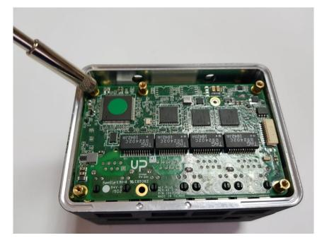
7. Place the bottom base on top of the NET Plus housing and tighten this with the M2.5\*4 screws which are reserved at first step.
