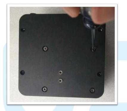
10. Fasten the bottom plate with top cover by screws x 4pcs
