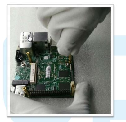
8. Place the board into the middle case, check well with the 4 sides exactly that match the IO sides.
