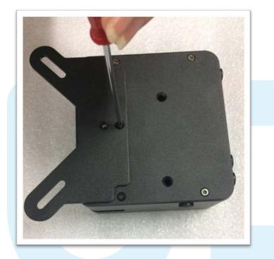
11. Fasten the Vesa Mount with pre-assembled case by screws x 2pcs
