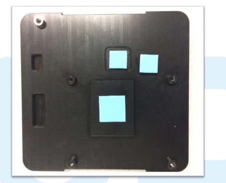
3. Peel of the blue protection film of thermal pad
