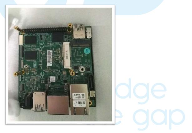
7. Fasten the PCB with top cover by the hex standoffs through the threads nut on the top cover.
