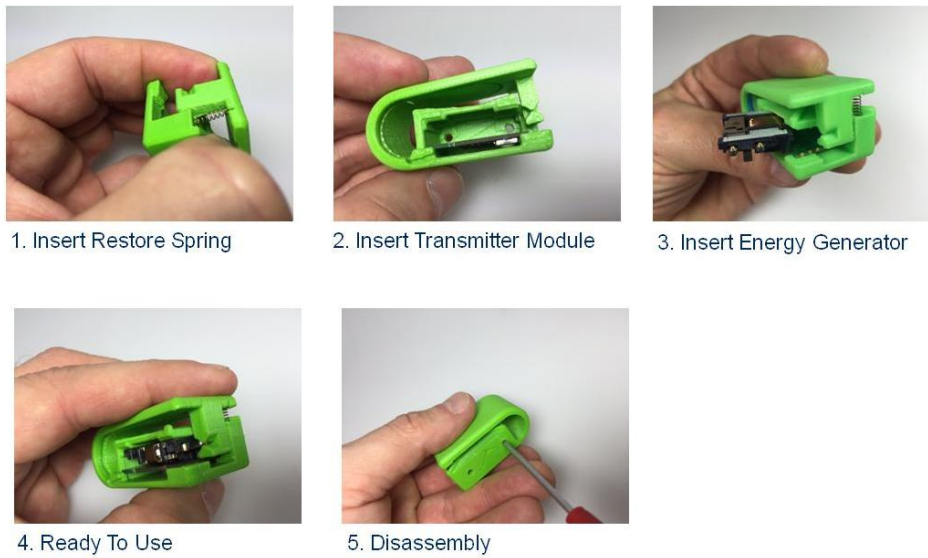
Figure 11: Clamp Switch – Assembly/Disassembly
