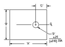
Thermasil III electrically insulating pad for a TO-220 device. Composed of a silicone elastomer binder with a thermally conductive filler and reinforced with finely woven glass cloth to resist tearing.
