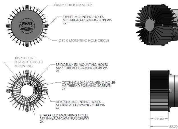
NOTE: DIN 7500 TYPE THREAD-FORMING SCREWS ARE RECOMMENDED FOR ALL MOUNTING HOLE BOSSES
