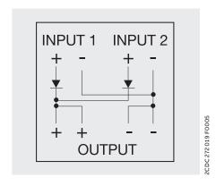
INPUT 1 +, - Connection of the output of power supply unit 1
