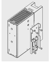
To mount the power supply in position 7 remove the DIN rail adapter that is fasten with 4 screws and attach it on the side of the power supply.
