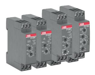
The CT-C range combines lower cost with higher value and performance by offering essential functions in a 17.5 mm housing, freeing up room in any control cabinet. The range includes 11 devices, offering both single and multifunctional types, with a time range from 0.05 seconds to 100 hours.
