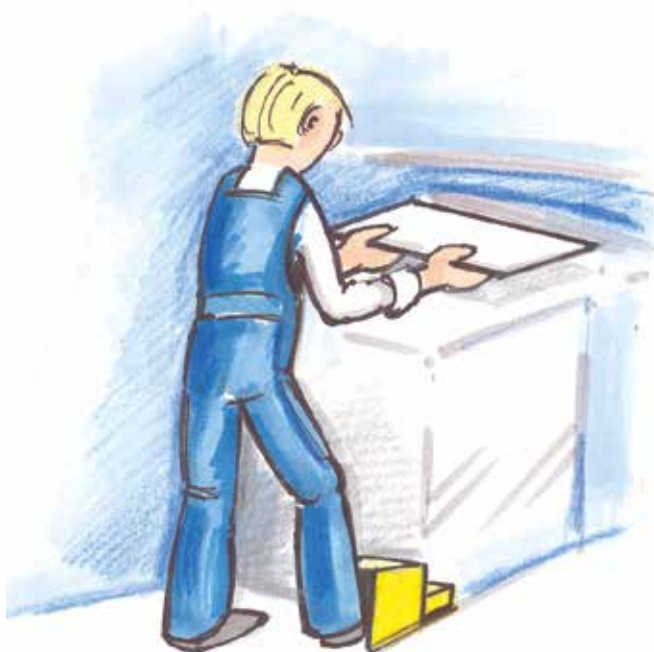
Safety foot operated switch with three-position function.
