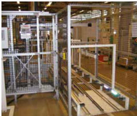
Quick-Guard Standard assembled with mesh.
