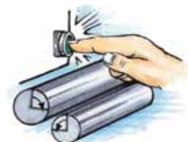
Shaft only turns a small amount each time the PB is pressed.
