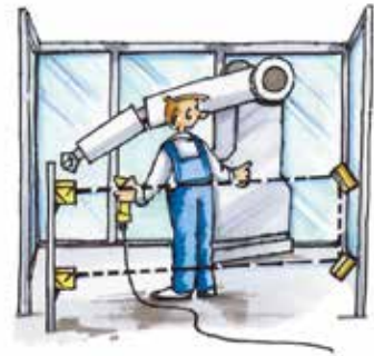
Light beam being bypassed for a maximum pre-set time e.g. 5 sec. by the jsht1 during entrance and exit with the JSHD4 Three Position Enabling device.
