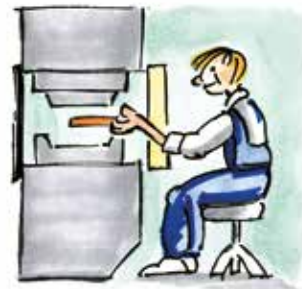
Light curtain to protect during cycle initiation
