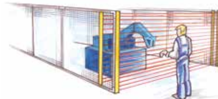
Light curtain for inner area limiting
