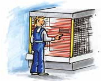
Resolution for finger ( \leq 14 mm) gives C = 0
