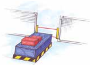
Light grids with monitored by-passing during material transport
