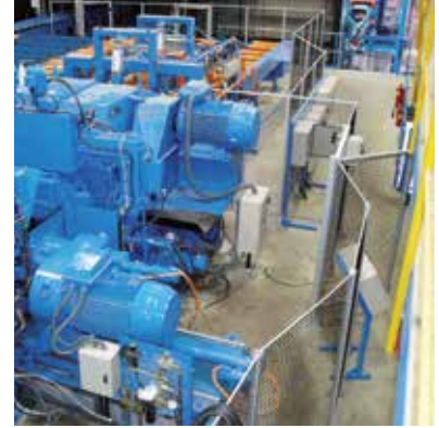
Quick-Guard Express with few components and easy to angle at up to 45°.
