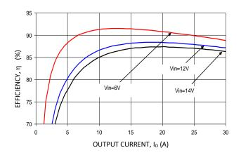
Figure 7. Converter Efficiency versus Output Current.
