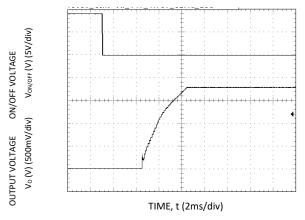
Figure 17. Transient Response to Dynamic Load Change from 0% to 50% to 0% with  $V_{\rm IN}$ =12V.
