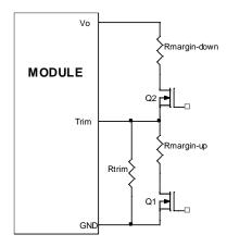
Figure 32. Circuit Configuration for margining Output voltage.
