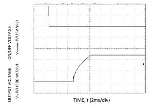
Figure 9. Typical Start-up Using On/Off Voltage (Io = Io,max).
