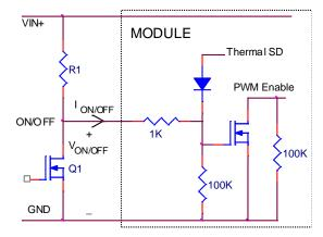
Figure 30. Remote On/Off Implementation using ON/OFF .
