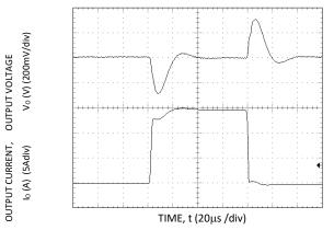
Figure 20. Typical output ripple and noise (V<sub>IN</sub> = 12V,  $I_0$  = 30A,  $C_{OUT}$  = 0.1 $\mu$ F // 47  $\mu$ F ceramic capacitors).
