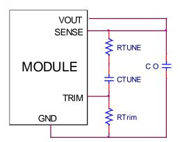
Figure. 34. Circuit diagram showing connection of  $R_{\text{TUME}}$  and  $C_{\text{TUNE}}$  to tune the control loop of the module.
