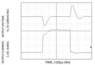
Figure 11. Transient Response to Dynamic Load Change from 0% to 50% to 0% with  $V_{\text{IN}}$ =12V.
