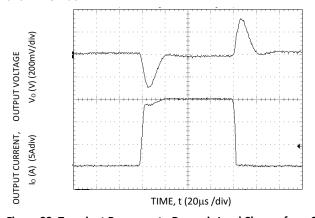
Figure 20. Typical output ripple and noise ( $V_{IN}$  = 12V,  $I_0$  = 30A,  $C_{OUT}$  = 0.1 $\mu$ F // 47  $\mu$ F ceramic capacitors).
