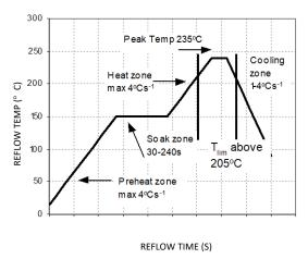
Figure 38. Reflow Profile for Tin/Lead (Sn/Pb) process.
