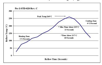
**NOTE:** Soldering outside of the recommended profile requires testing to verify results and performance.
