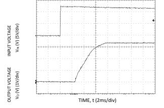
Figure 21. Typical Start-up Using On/Off Voltage (Io = Io,max).
