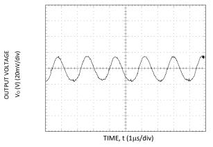
Figure 8. Typical output ripple and noise ( $V_{IN} = 12V$ ,  $I_0 = 30A$ ,  $C_{OUT} = 0.1 \mu F$  // 47  $\mu F$  ceramic capacitors ).
