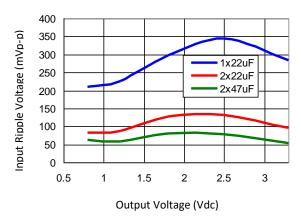
Figure 28. Input ripple voltage for various output voltages with 1x22  $\mu$ F, 2x22  $\mu$ F or 2x47  $\mu$ F ceramic capacitors at the input (30A load). Input voltage is 12V.
