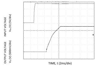
Figure 15. Typical Start-up Using On/Off Voltage (Io = Io,max).
