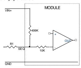
Figure 33. Circuit showing connection of the sequencing signal to the SEQ pin.
