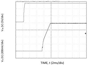
Figure 3. Typical Start-up Using On/Off Voltage (Io = Io,max).
