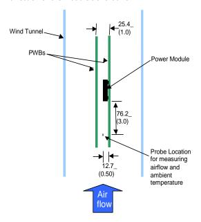
Figure 35. Thermal Test Setup.
