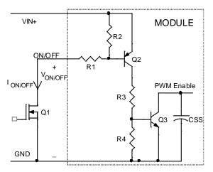
Figure 28. Circuit configuration for using positive logic On/OFF.
