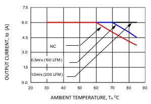
Figure 19. Derating Output Current versus Local Ambient Temperature and Airflow (Vin = 5.0, Vo=3.3Vdc).
