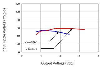
Figure 27. Input ripple voltage for various output with 2x150  $\mu$ F polymer and 2x47  $\mu$ F ceramic capacitors at the input (80% of Io,max).
