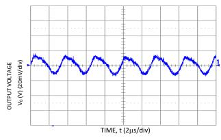
Figure 9. Typical Output Ripple and Noise (Vin = 5.0V dc, Vo = 3.3 Vdc, Io=6A).
