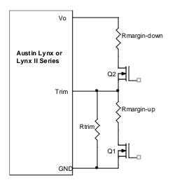
Figure 31. Circuit Configuration for margining Output voltage.
