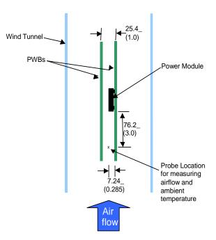
Figure 33. Thermal Test Set-up.
