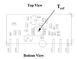
Figure 32. Tref Temperature measurement location.
