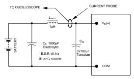
NOTE: Measure input reflected ripple current with a simulated source inductance ( $L_{TEST}$ ) of 1 $\mu$ H. Capacitor  $C_S$  offsets possible battery impedance. Measure current as shown above.
