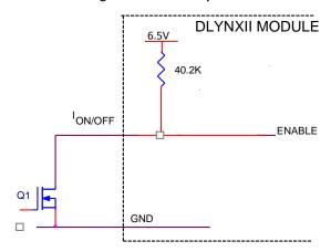
Figure 39. Circuit configuration for using positive On/Off logic.
