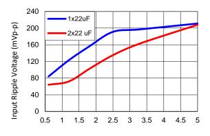
Figure 37. Input ripple voltage for various output voltages with 1x22  $\mu$ F or 2x22  $\mu$ F ceramic capacitors at the input (4A load). Input voltage is 12V.
