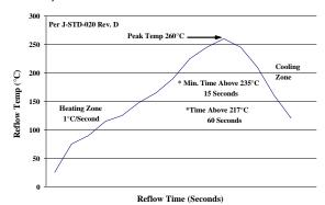
Figure 50. Recommended linear reflow profile using Sn/Ag/Cu solder.
