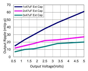
Figure 38. Output ripple voltage for various output voltages with external 1x47  $\mu$ F, 2x47  $\mu$ F or 3x47  $\mu$ F ceramic capacitors at the output (4A load). Input voltage is 12V.
