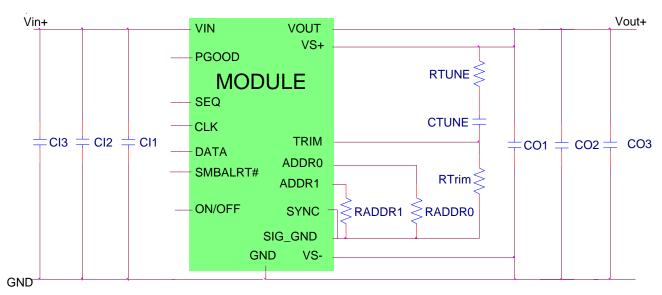
Cl1 Decoupling cap - 1x0.047µF/16V ceramic(e.g. Murata LLL185R71C473MA01) + 1x0.1uF/16V 0402 ceramic
