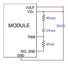
Figure. 46. Circuit diagram showing connection of  $R_{\text{TUME}}$  and  $C_{\text{TUNE}}$  to tune the control loop of the module.
