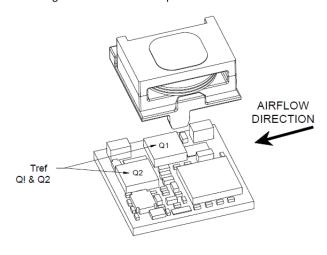
Figure 49. Preferred airflow direction and location of hotspot of the module (Tref).
