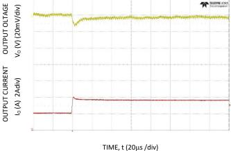
Figure 3. Typical output ripple ( $C_0$ =3x22 $\mu$ F ceramic,  $V_{IN}$  = 12V,  $I_0$  = Figure 4. Transient Response to Dynamic Load Change from 50% to  $I_{O,max}$ ,).
