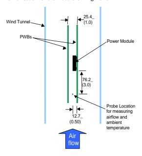
Figure 48. Thermal Test Setup.
