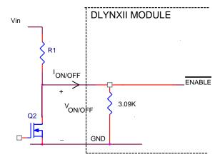
Figure 40. Circuit configuration for using negative On/Off logic.
