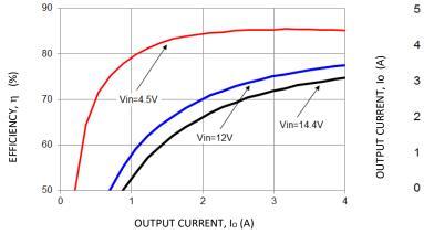
Figure 1. Converter Efficiency versus Output Current.
