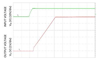
Figure 35. Typical Start-up Using On/Off Voltage (Io = Io,max).
