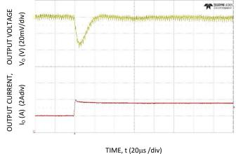
Figure 15. Typical output ripple and noise (C<sub>O</sub>=3X22μF ceramic, V<sub>IN</sub> Figure 16. Transient Response to Dynamic Load Change from 50% to = 12V, I<sub>O</sub> = I<sub>O,max</sub>, ). 100% at 12Vin, Cout=5x47uF, CTune=4.7nF, RTune=300
