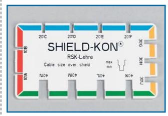
The choice of the appropriate connector and die set mainly depends on the size of the shielded cable. The selection can be done very quickly with the RSK-LEHRE gauge.
