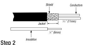
Select the appropriate connector according to the size of the shielded cable (see **page G-80**). Place the ground wire around the trap hook and the shielded wire into the bottom of the connector.
