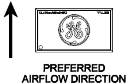
Figure 50. Preferred airflow direction and location of hot-spot of the module ( T_{ref} ).
