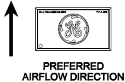
Figure 48. Preferred airflow direction and location of hot-spot of the module ( T_{ref} ).
