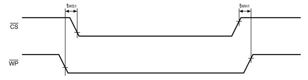
Figure 7 Valid Timing in Write Protect
