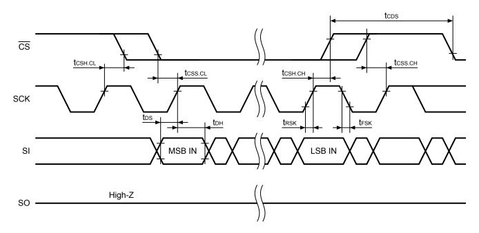
Figure 4 Serial Input Timing
