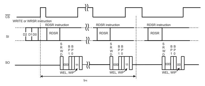
Figure 10 Usage Example of WEL, WIP Bits during Write
