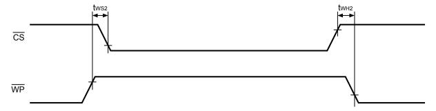
Figure 8 Invalid Timing in Write Protect
