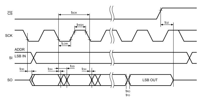
Figure 6 Serial Output Timing
