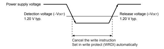
Figure 19 Operation during the Low Power Supply Voltage
