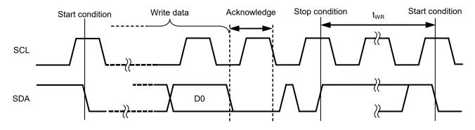
Figure 3 Write Cycle Timing
