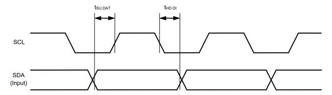
Figure 5 Data Transmission Timing
