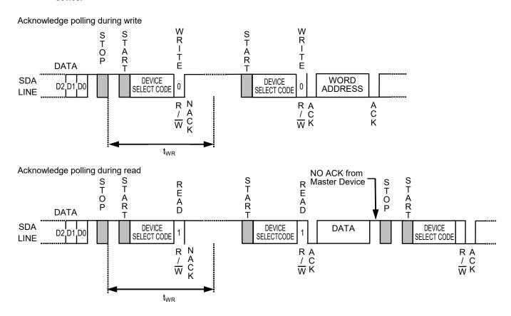
**Remark** Users are able to input data after acknowledge output in acknowledge polling during write. Users are able to read data after acknowledge output in acknowledge polling during read.
