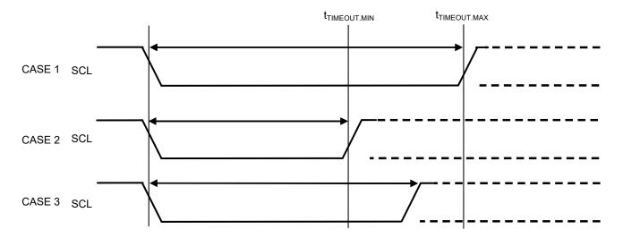
CASE1: SCL clock time "L" (t<sub>LOW</sub>) ≥ t<sub>TIMEOUT.MAX</sub>, this IC will reset the bus communication and return to standby mode.
