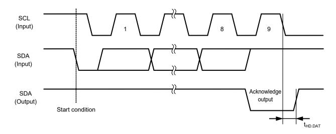
Figure 6 Acknowledge Output Timing
