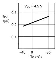
2. 8 Data output delay time t<sub>PD</sub> vs. ambient temperature Ta
