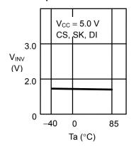
1. 31 Low supply voltage detection voltage -V<sub>DET</sub> vs. ambient temperature Ta
