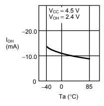
1. 20 High-level output voltage V<sub>OH</sub> vs. ambient temperature Ta
