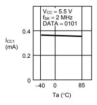
1. 2 Current consumption (READ) I<sub>CC1</sub> vs. ambient temperature Ta
