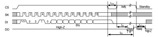
Figure 10 Chip Erase Timing
