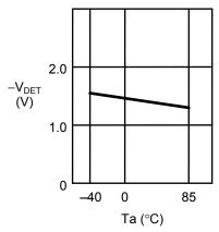
1. 32 Low supply voltage release voltage +V<sub>DET</sub> vs. ambient temperature Ta
