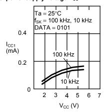
1. 6 Current consumption (READ) I<sub>CC1</sub> vs. Clock frequency f<sub>SK</sub>
