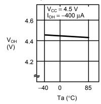
1. 18 High-level output voltage V<sub>OH</sub> vs. ambient temperature Ta
