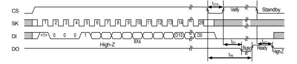
Figure 9 Chip Write Timing
