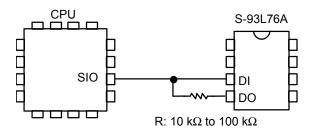
Figure 13 Connection of 3-Wire Interface
