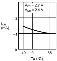
1. 25 High-level output current lon vs. ambient temperature Ta
