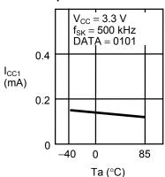
1. 3 Current consumption (READ) I<sub>CC1</sub> vs. ambient temperature Ta
