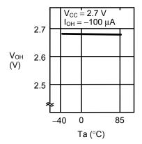
1. 19 High-level output voltage V<sub>OH</sub> vs. ambient temperature Ta
