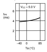
2. 4 Write time t<sub>PR</sub> vs. ambient temperature Ta
