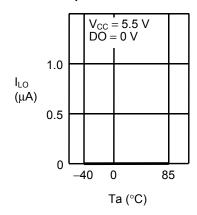
1. 16 Output leakage current I<sub>LO</sub> vs. ambient temperature Ta
