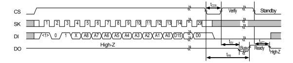
Figure 7 Data Write Timing
