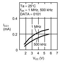
1. 5 Current consumption (READ) I<sub>CC1</sub> vs. power supply voltage V<sub>CC</sub>
