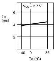
2. 7 Data output delay time t<sub>PD</sub> vs. ambient temperature Ta
