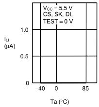
1. 14 Input leakage current I∟ vs. ambient temperature Ta
