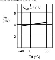
2. 5 Write time t<sub>PR</sub> vs. ambient temperature Ta
