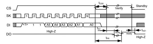
Figure 6 Data Erase Timing (S-93S46A)
