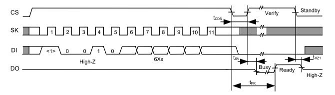
Figure 11 Chip Erase Timing (S-93S56A/66A)
