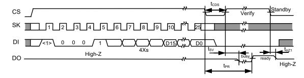
Figure 8 Chip Write Timing (S-93S46A)
