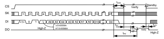
Figure 5 Data Write Timing (S-93S56A/66A)
