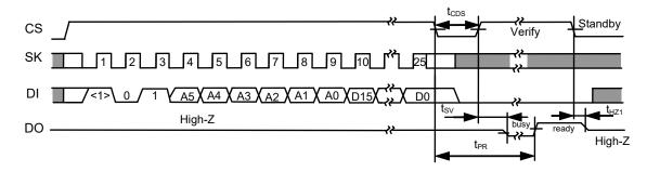
Figure 4 Data Write Timing (S-93S46A)
