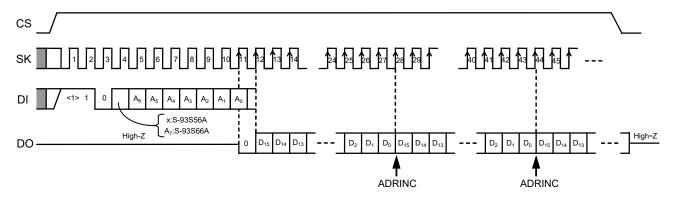
Figure 3 Read Timing (S-93S56A/66A)
