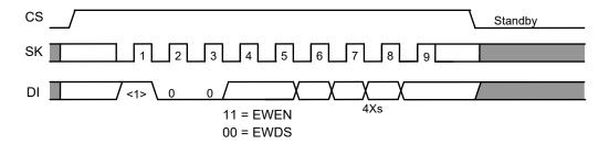
Figure 12 Write Enable / Disable Timing (S-93S46A)
