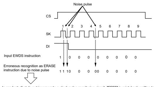
In products that do not incorporate a clock pulse monitoring circuit, "FFFF" is mistakenly written to address 00h. However the S-93S46A detects the overcount and cancels the instruction without performing a write operation.
