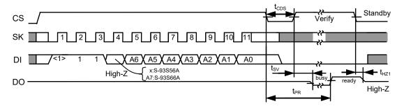
Figure 7 Data Erase Timing (S-93S56A/66A)
