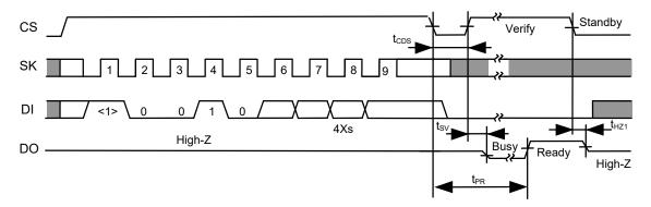
Figure 10 Chip Erase Timing (S-93S46A)
