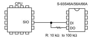
Figure 17 Connection of 3-Wire Interface
