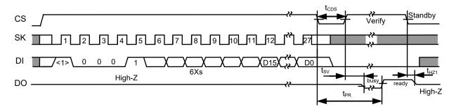
Figure 9 Chip Write Timing (S-93S56A/66A)
