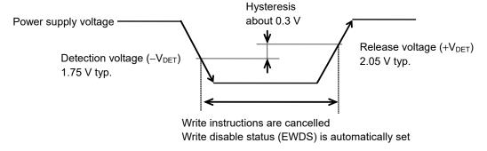
Figure 14 Operation during the Low Power Supply Voltage
