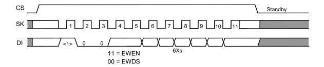
Figure 13 Write Enable / Disable Timing (S-93S56A/66A)
