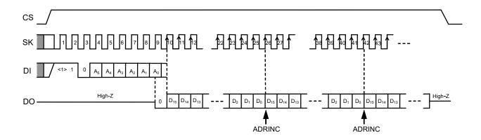
Figure 2 Read Timing (S-93S46A)
