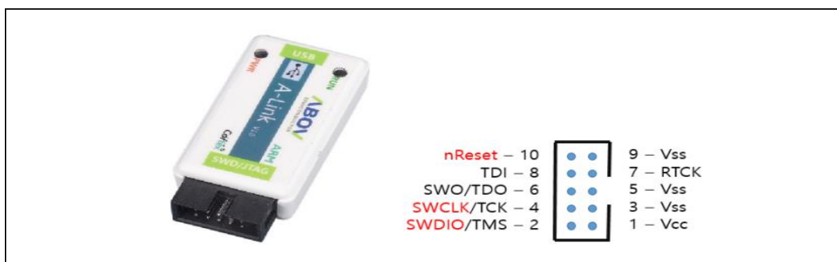
Figure 55. A-Link and Pin Descriptions
