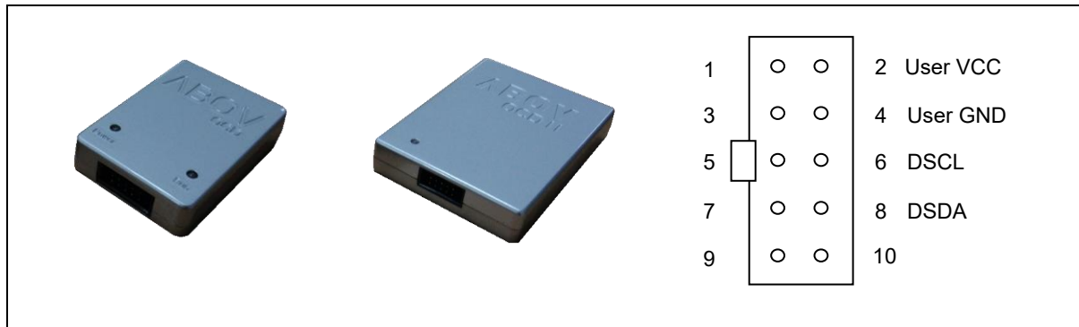
Figure 42. Debugger (OCD1/OCD2) and Pinouts
