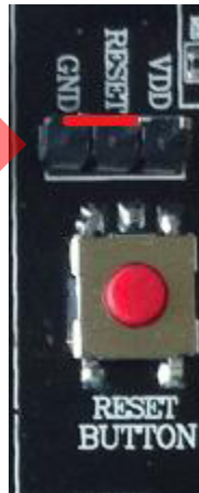
Figure 9: Jumper setting for low effective RESET
