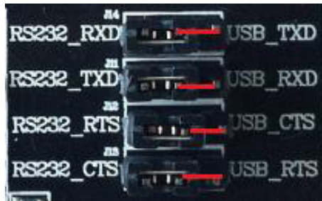
Figure 5: USB to serial jumper connect
