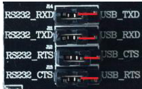
Figure 5: USB to serial jumper connect
