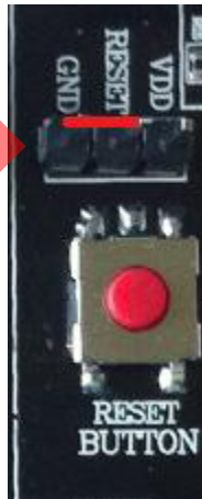
Figure 9: Jumper setting for low effective RESET
