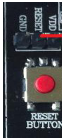
Figure 8: Jumper setting for high effective RESET
