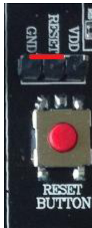
Figure 9: Jumper setting for low effective RESET
