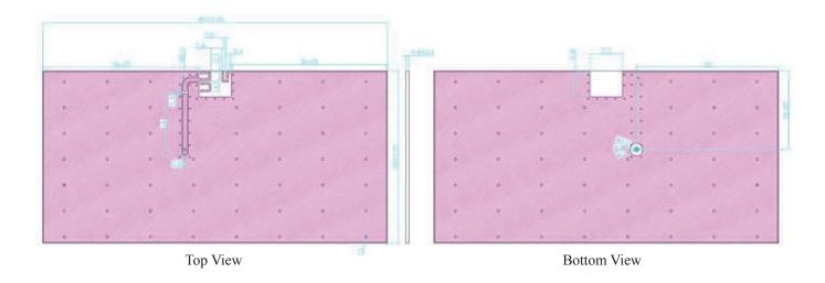
Evaluation Board dimension: 80 x 40 mm Unit: mm
