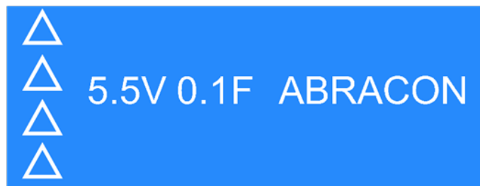
Example of the Markings of a 5.5V 0.1F supercapacitor
