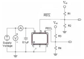
Vdd= 3.3V: R1=R3=127Ω; R2=R4=82.5ΩVdd= 2.5V: R1=R3=250Ω; R2=R4=62.5Ω
