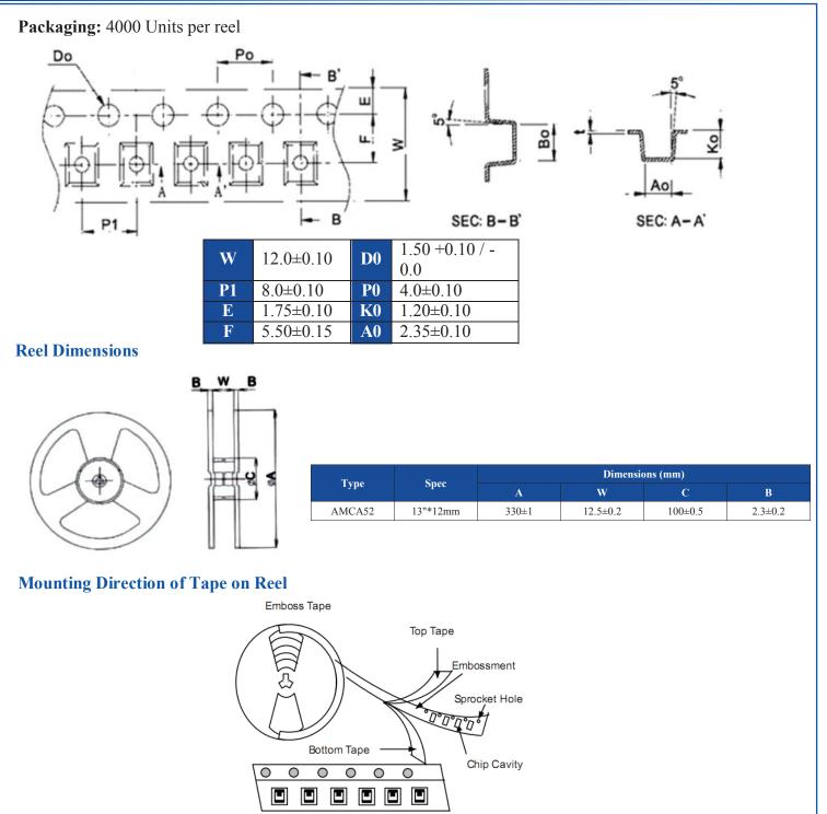
Note: The sprocket holes are to the right as the tape is pulled toward the user.
