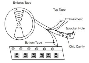
Note: The sprocket holes are to the right as the tape is pulled toward the user.
