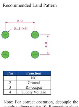
Note: For correct operation, decouple the supply voltage with a  $10\mu$ F capacitor close to the oscillator.
