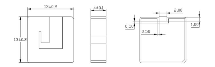
Unit: mm General Tolerance: ±0.3mm
