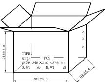
The GPS antenna 50 pcs are packed per tray, 5 trays are packed per vacuum bag, 4 vacuum bags per carton, and 1000 pcs GPS antenna per carton. The size of each carton is 345\*210\*275mm.
