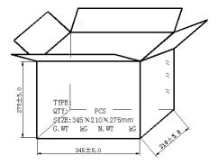
The GPS antenna 50 pcs are packed per tray, 5 trays are packed per vacuum bag, 4 vacuum bags per carton, and 1000 pcs GPS antenna per carton. The size of each carton is 345\*210\*275mm.
