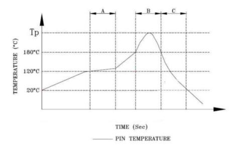
A. Preheating B. Soldering C. Gradual Cooling
