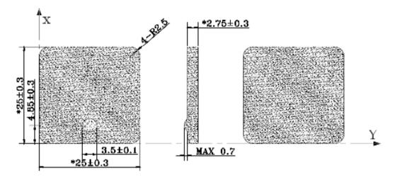
Mounting: The antenna is mounted with double sided adhesive tape that is attached to the underside of the antenna.
