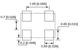
Note: Recommend using an approximately 0.01uF bypass capacitor between PIN 2 and 4.
