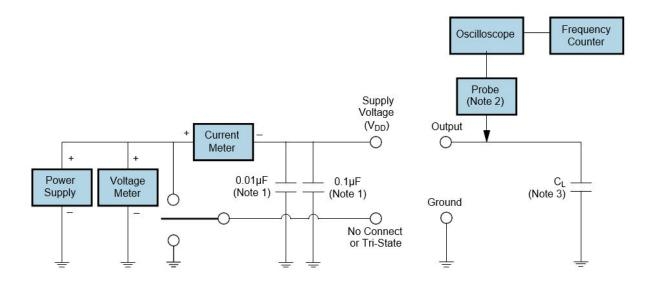
**Note 1:** An external 0.1µF low frequency tantalum bypass capacitor in parallel with a 0.01µF high frequency ceramic bypass Capacitor close to the package ground and VDD pin is required.
