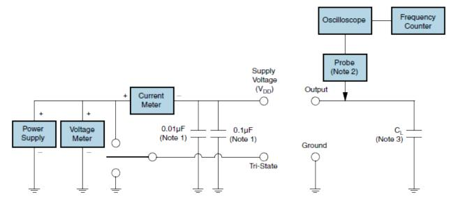
Note 1: An external 0.1μF low frequency tantalum bypass capacitor in parallel with a 0.01μF high frequency ceramic bypass Capacitor close to the package ground and supply voltage pin is required.
