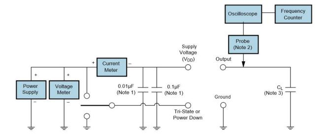
Note 1: An external 0.01µF ceramic bypass capacitor in parallel with a 0.1µF high frequency ceramic bypass capacitor close (less Than 2mm) to the package ground and supply voltage pin is required.
