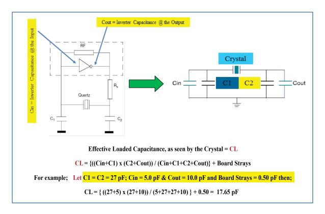
Therefore specifying a crystal with 18.0 pF plating load capacitance would be the closest match for frequency accuracy.
