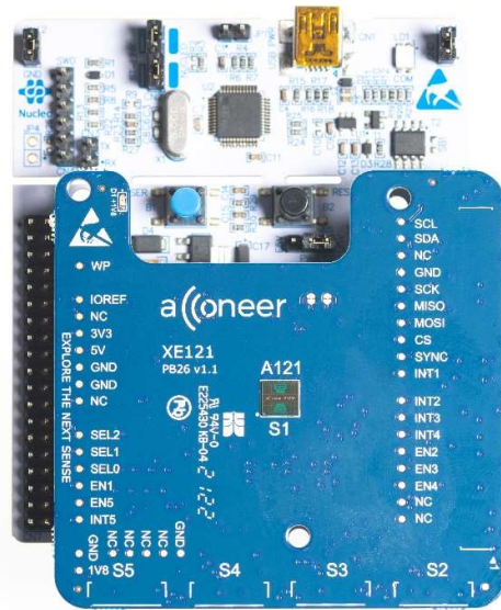
Picture 6. XE121 connected to an STM Nucleo Development Board.
