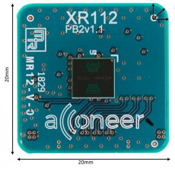
x=y=2.05mm r = 2.9mm PCB thickness: 0.9mm
