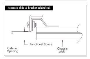
The drawings at left show several mounting configurations from an overhead perspective. This viewpoint demonstrates how chassis widths are calculated; slide thickness evaluated, and installations of brackets verified.
