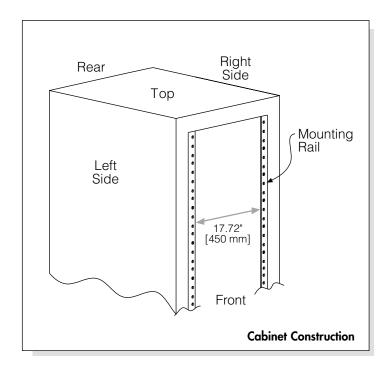
Most electronic cabinets/enclosures are based on dimensional guidelines as illustrated in the ANSI/EIA 310 Specifications.
