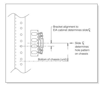
In other situations, one element of the slide installation is known and this determines slide positioning.
